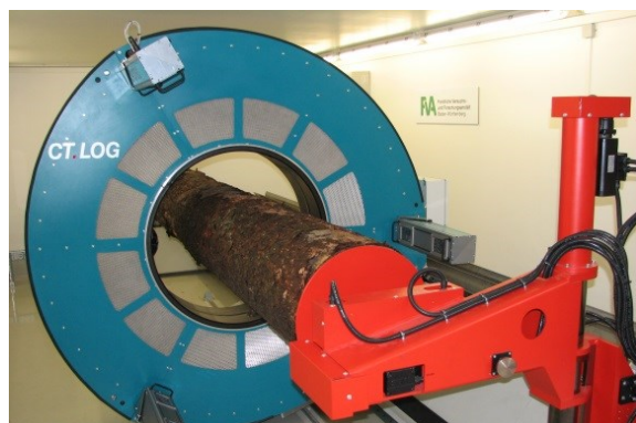
Computer Tomograph CT.LOG at FVA; Photo: A. Püschel
